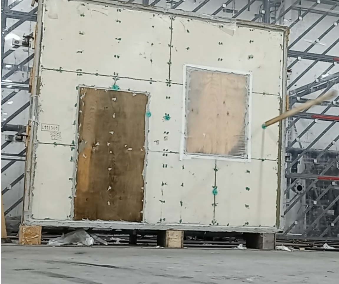
Photo No. 2 Specimen #4 Large Missile Impacts
